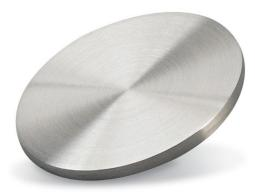
This article describes target material options for sputter coaters that deposit a thin metal coating on non-conductive SEM samples. Coating a sample with a conductive metal renders an insulating sample conductive enough to minimize charging effects on the SEM image. In most cases, coating SEM samples with only a few nanometres of a metal results in crisp, clear images. Proper target material selection is dictated by overall imaging requirements, the SEM available, the
